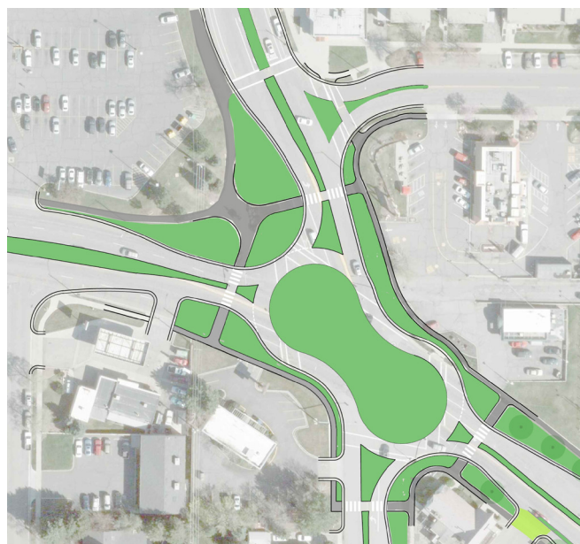
Option C: Concept diagram of a roundabout at 2300 East
